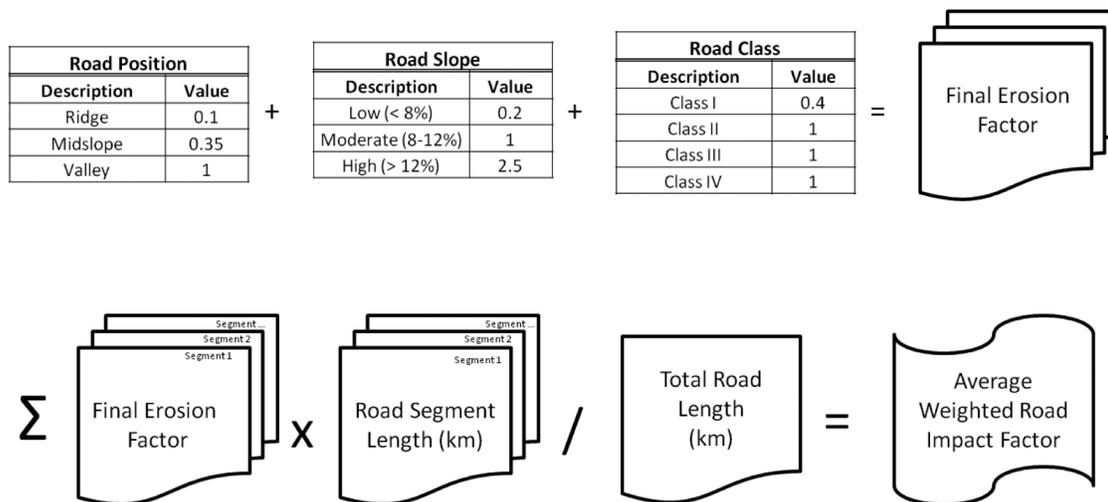
Figure 3—Flowchart of final erosion factor and final watershed road impact factor. Adapted from Bernard (2006).
