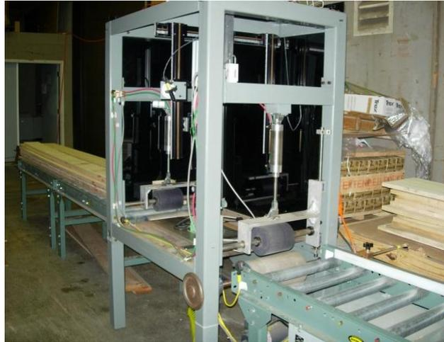
Figure 1. A prototype scanning system for hardwood lumber. This was originally designed to detect wane and surface defects in unplanned boards.
